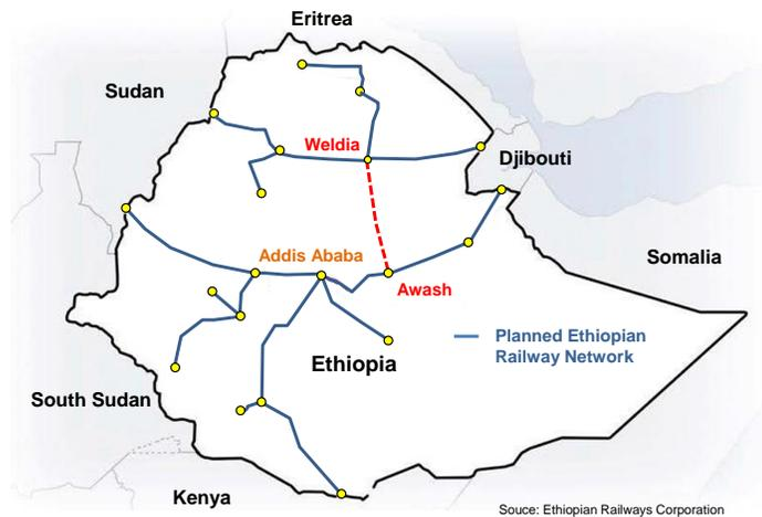
The new railway line between Awash and Weldia comprises the construction of approx. 389 km new electrified railway line, approx. 40 km maintenance and approx. 18 km station lines. It also includes construction of new tunnels, railway stations, maintenance and workshop facilities, depots and necessary signalling and power supply infrastructure.
